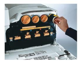
Loading toners is a clean and simple process, easily done from the front of the printer.
