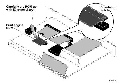
**Note** Identify Pin 1 end of the adaptor board the square pads on the upper surface of the board; alternately, you can identify the pin 1 end by the notch in the pin array on the bottom-side of the board. Likewise, a notch on the end of the ROM IC chip indicates the pin 1 end of the chip.
