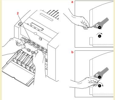
b To clean the upper rubber rollers, place and hold an alcohol-soaked swab against the underside of each roller while turning the lower roller shaft with your thumb and forefinger. **Scrub each roller thoroughly.** You'll need several swabs to clean the rollers. When the swab becomes dirty during cleaning, discard it and use another.
