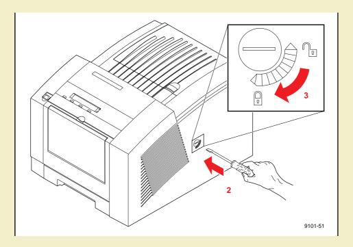
While pressing inward with medium pressure, turn the transit restraint slot in a *clockwise* direction to lock the printhead in position. The lock button is recessed from the side of the printer when fully engaged.
