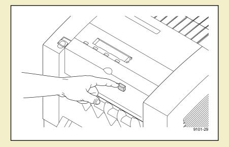
4 Using both hands, pull the jammed media out the top of the printer.
