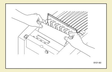
5 If necessary, remove the media tray to locate and clear jammed media.
