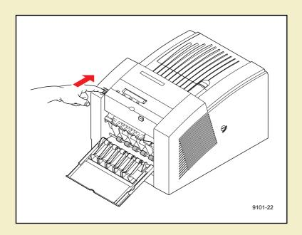
If necessary, open the exit cover using the blue release button located inside the front cover, at the top of the printer.
