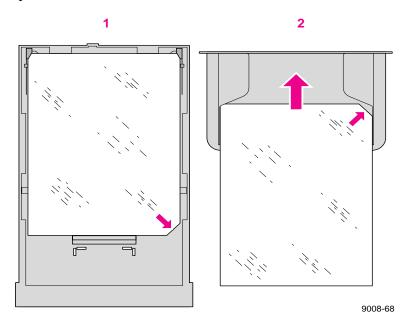
Note Do not re-use transparencies that have been fed through the printer once, for example, after jams or if the transparency is ejected without being printed; you may damage the printer.
