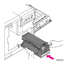
**4.** Lock the fuser by turning the **small** blue screw *clockwise* several turns.
