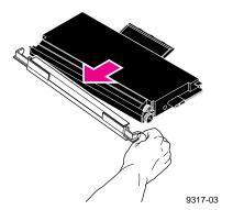
4. Insert the toner cartridge in the slot labeled for its color.
